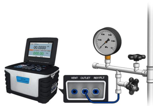
Figure 3-20 Calibrating a dial pressure gauge
