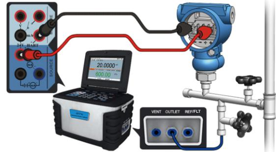
Figure 3-22 Calibrating a two-wire pressure transmitter
