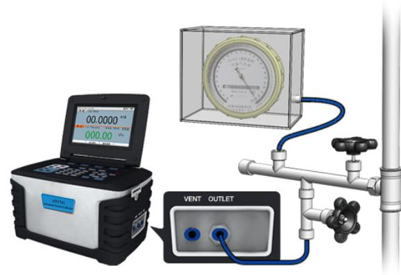
Figure 5-3 Calibrating an aneroid barometer
