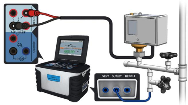
Figure 3-18 Calibrating a pressure switch
