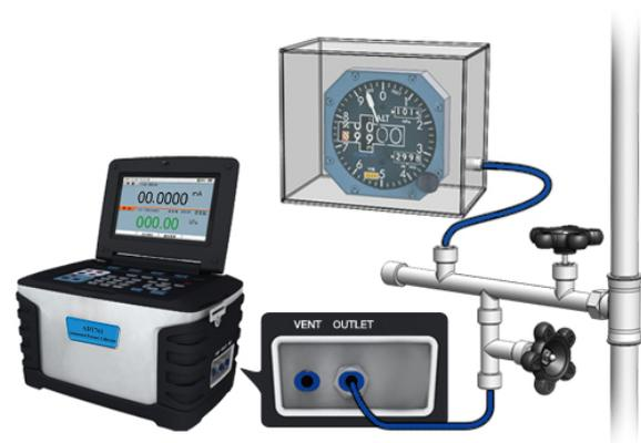
Figure 5-4 Calibrating a barometer altimeter
