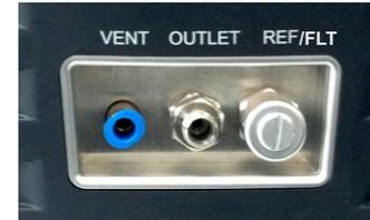
Figure 2-7 Pneumatic connection
