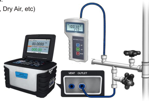
Figure 5-1 Calibrating a digital barometer
