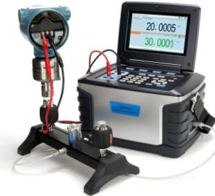
Figure 3-3 Gauge pressure source
