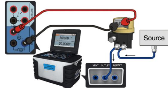
Figure 3-19 Calibrating a I/P converter
