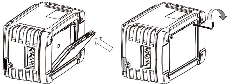
Figure 2-4 Battery installation
