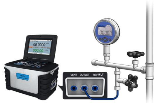
Figure 3-21 Calibrating a digital pressure gauge
