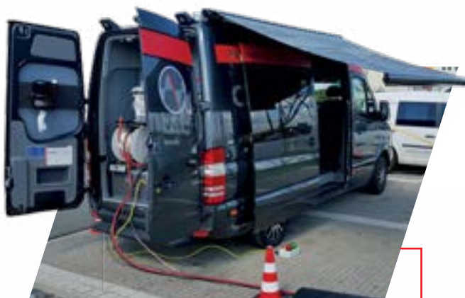
Cable test and fault location
